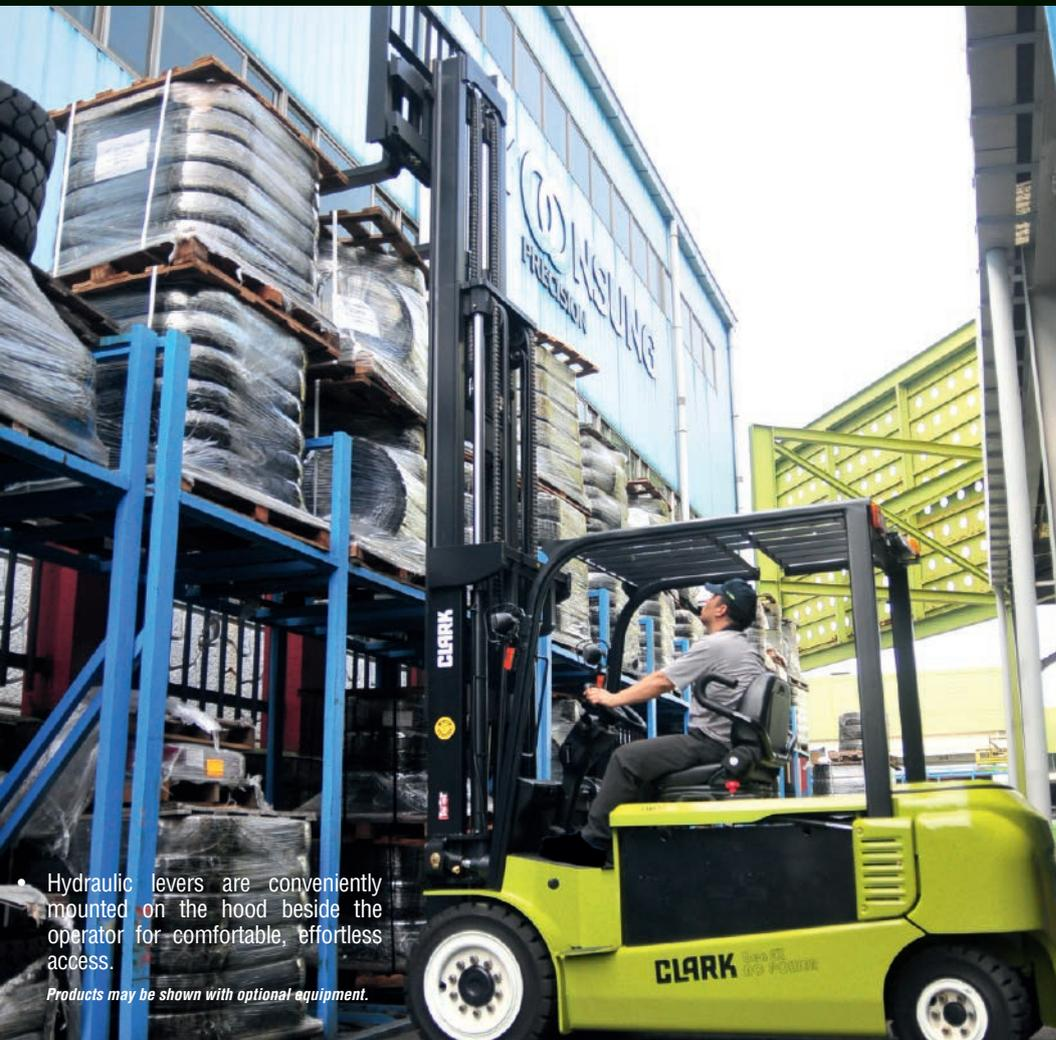
• Hydraulic levers are conveniently mounted on the hood beside the operator for comfortable, effortless access.
