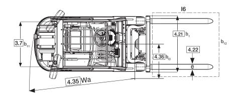
$$\begin{split} &A_{st} = \ Wa + x + I_6 + a \\ &\text{applies only if} \quad \frac{b_{12}}{2} < b_{13} \\ &A_{st} = \ Wa + \sqrt{(\ I_6 + x)^2 + \left(\frac{b_{12}}{2} - b_{13}\right)^2} + a \\ &\text{applies only if} \quad \frac{b_{12}}{2} \ge b_{13} \\ &a = 200 \end{split}$$
